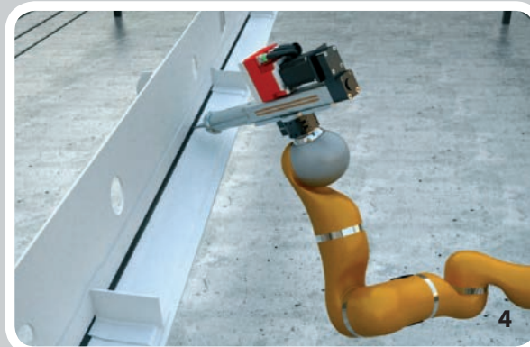
Exemplary sealant application on long part (over 3 m in length)
