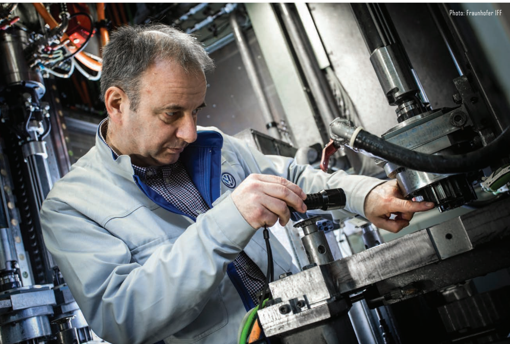
Jörg Rudolph, a specialist at VW, inspecting honing tools for damage.
