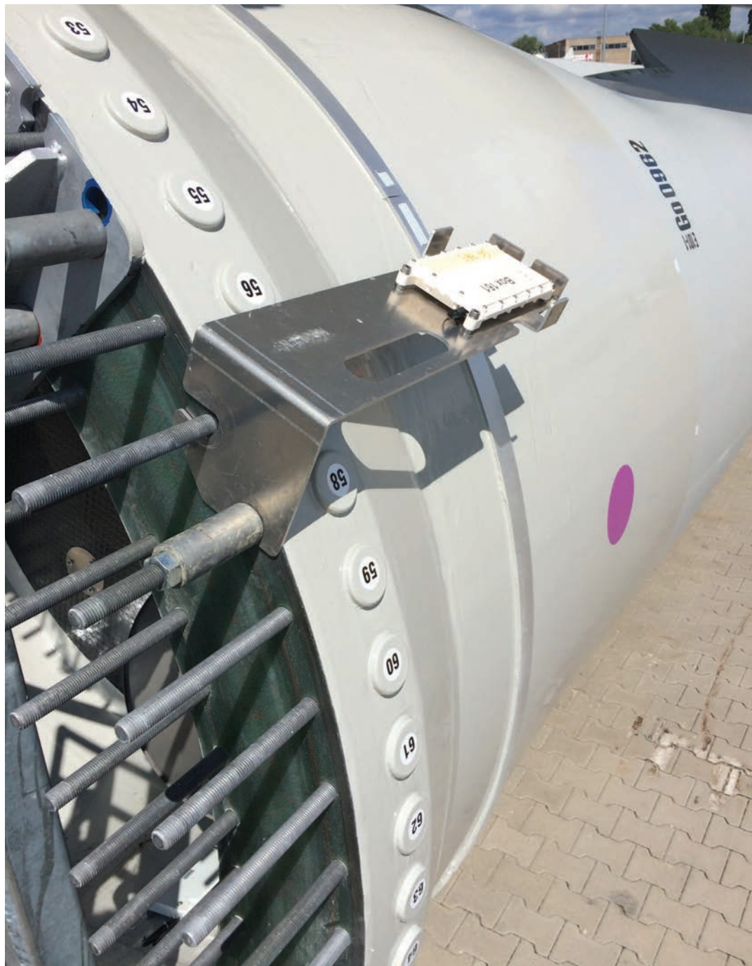
The RFID chip on a part contains its digital history record and transmits its location to the central server as soon as the part is moved.
