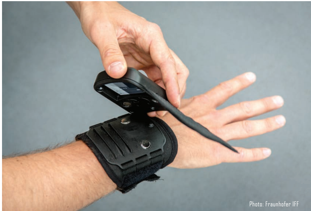
RFID wristband design and a wristband being put on.
