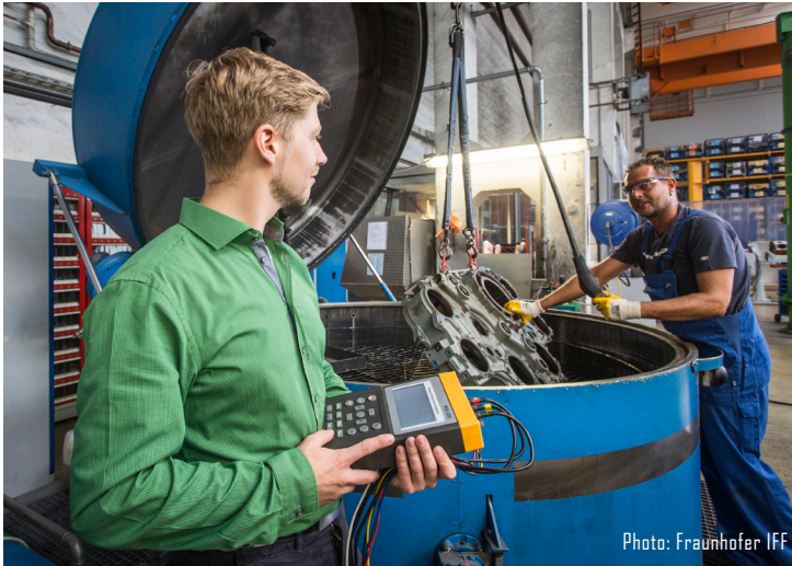
Equipped with portable measuring instruments, Fraunhofer researchers examined some thirty to forty machines more closely. The outcome was a time curve of power consumption and the compilation of an energy portfolio.
