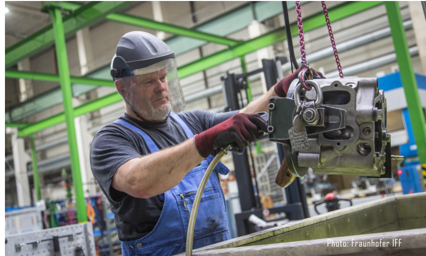
The sometimes up to over 1,000 components that make up an engine are cleaned and re-manufactured at MTU Reman to do their job again – virtually like new – in a remanufactured engine. The remanufacturing of cylinder heads particularly consumes a lot of energy.
