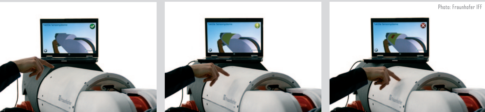
With the sensor skin, a robot not only senses that a person is approaching but also from what direction.
