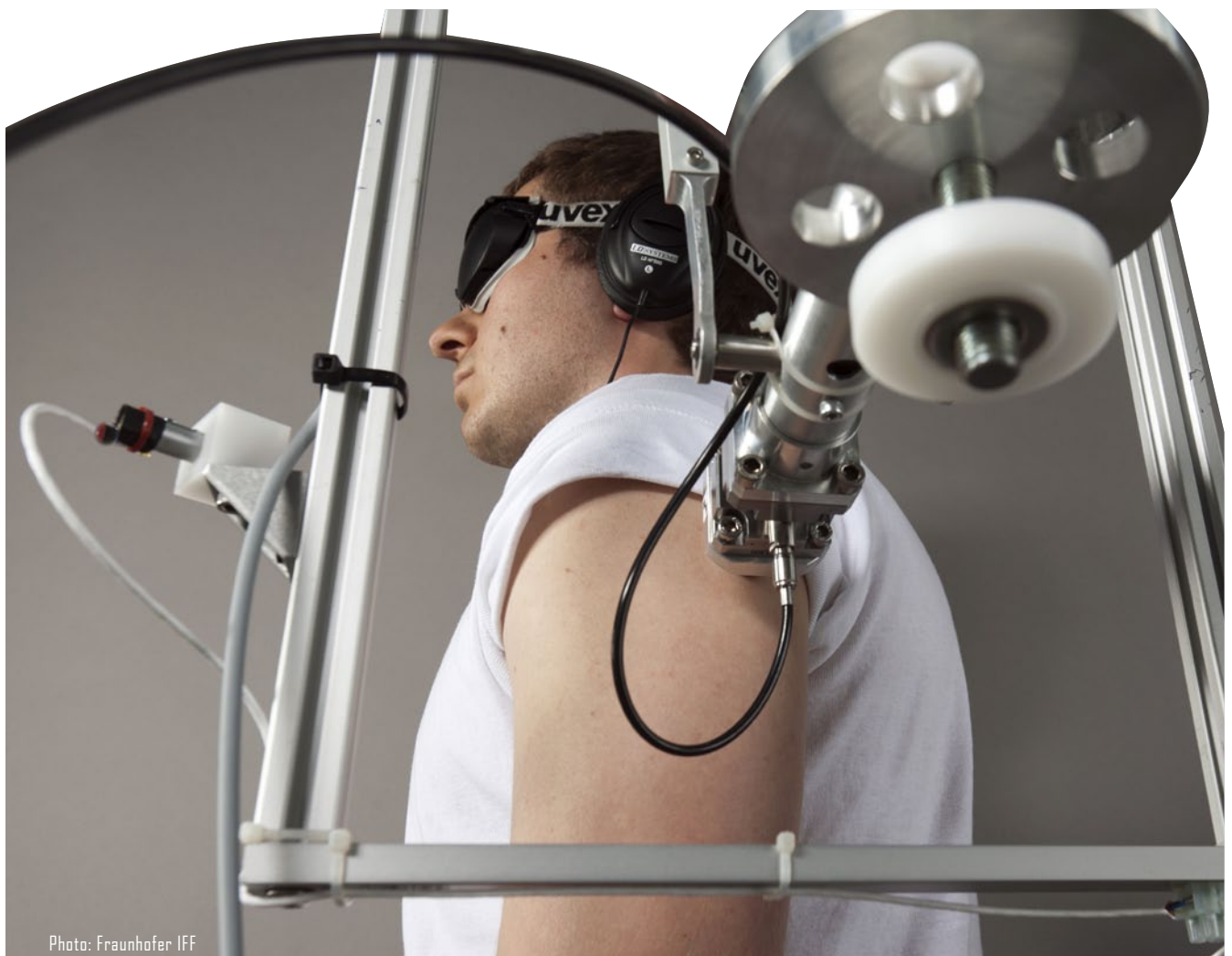
A subject during the study's impact test. How much force can act on a human body before a bruise appears?
