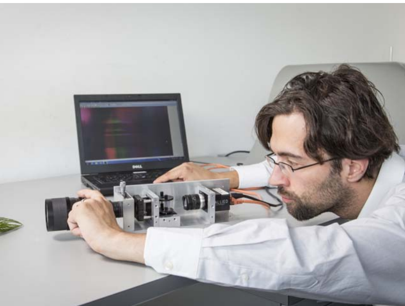
Hans-Christian Klück developed a small and flexible hyperspectral camera. The camera delivers an overview of many ingredients present in plants. Photos: Dirk Mahler
