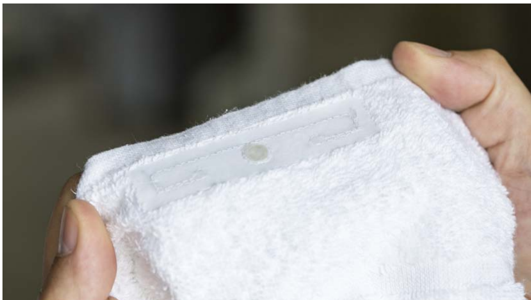
The special RFID chips hold up better in numerous wash cycles than laundry items. In the future, they will grow so small that they disappear in the seams of towels and bedsheets.
