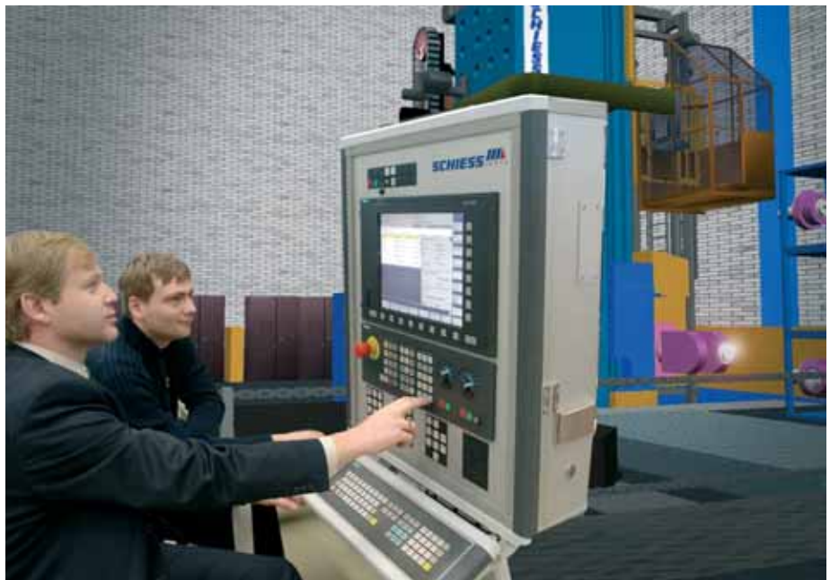
Figure 1: Connecting a CNC machine control with the virtual model of a heavy tool machine in an interactive 3-D environment.
