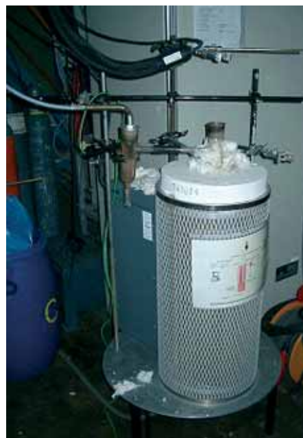
Figure 3: Lab fluidized bed reactor for testing OSEP measuring behavior.
