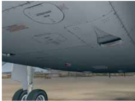
Figure 3: Detail of the underside of the nacelle with labeling, seals, rivets and diverse traces of wear.
