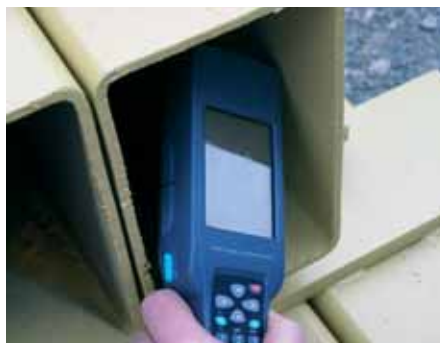
Figure 3: Mobile job management with RFID.
