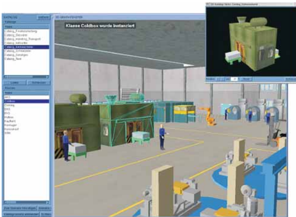
Figure 2: Modeling with the support of a library of predefined modules.
