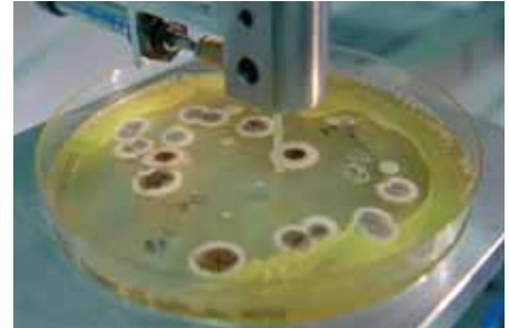
Figure 1: Automatic, sterile sampling from a fungus culture bred on culture agar as the growth medium in a Petri dish.
