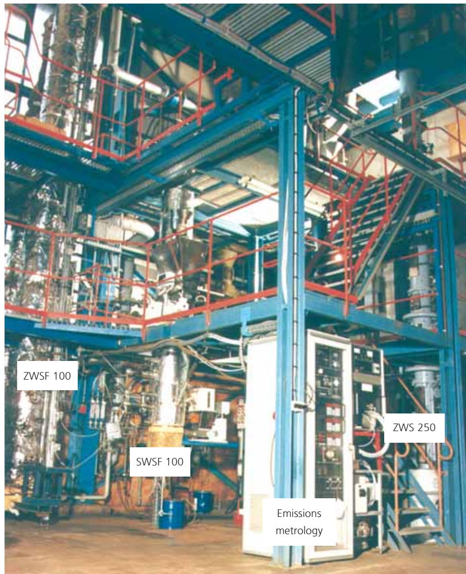
Figure 1: Experimental fluidized bed plants ZWSF 100, SWSF 100, ZWS 250 with gas emission metrology.
