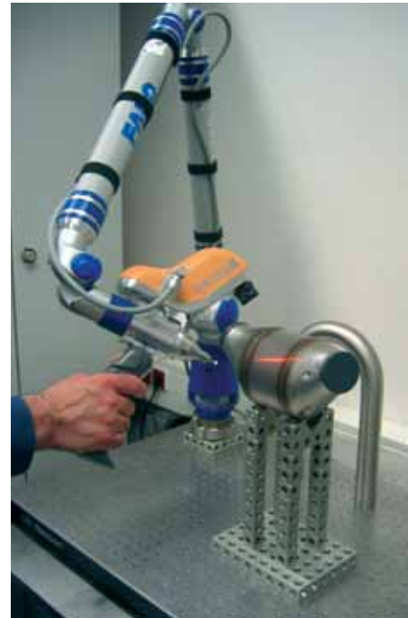
Figure 1: Manually guided measuring arm with light-sectioning sensor.
