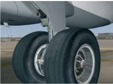
Figures 4 and 5: Examples of potential defects during the interactive walkaround: Extreme partial tire wear (left); collision damage on the radome covering (right).
