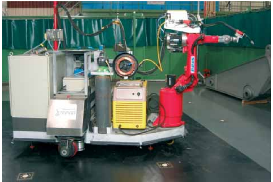
Figure 2: Full view of the autonomous, flexible robot for welding large steel structures.
