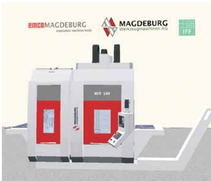
Figure 1: Virtual model of the vertical lathe MVT160 including its peripheral equipment.
