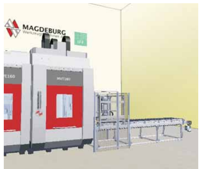
Figure 4: Configuration management makes it possible to represent the machine with various configurations, e.g. coupled with different storage solutions.
