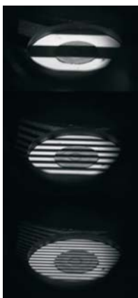
Figure 2: Rivet under coded illumination.
